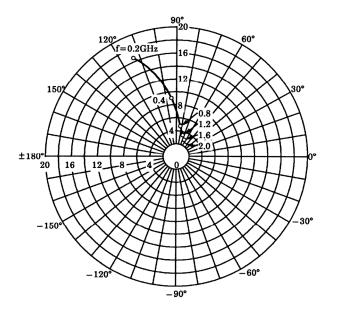
$\begin{array}{l} S_{12e} \\ V_{CE} = 10V \\ I_{C} = 20 \text{mA} \\ Ta = 25 ^{\circ}\text{C} \end{array}$
